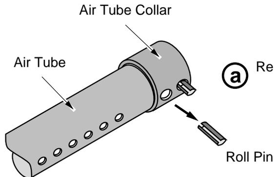
**a** Remove the left pin on the air tube collar
