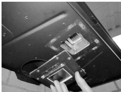
3. Pull down the upper accent light enclosure from the roof of the firebox, as shown below. Note the 3 screws holding the bulb assembly in place.
