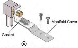
Apply thread sealant to the LP orifices prior to installation. Use the chart in the "Gas Specifications" section to determine the correct orifices.
