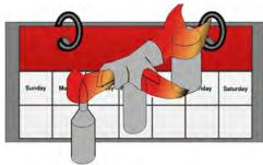
When in CPI mode the pilot will remain lit as long as the burner is engaged within a 7-day window. Each time the burner is turned on the 7-day timer resets. If the burner is not engaged within the 7-day window, the pilot will automatically revert to IPI mode and turn off to conserve fuel.
