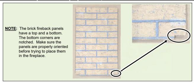
4. Tilt one of the side firebacks and place it inside the fireplace. Set the bottom edge of the fireback panel up against the bottom of the side wall of the firebox (there is a channel on the floor of the firebox that the fireback sets in). Tilt the top edge of the fireback up until the fireback is tight against the side wall of the fireplace. Replace the (2) fireback clips to secure the fireback in place. Repeat this process for the opposite side fireback.
