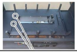
**NOTE:** When reinstalling the center burner make sure that the holes on the left end of the burner engage the two locating pins.
