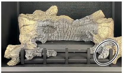
Install log #6 as shown below. The hole in the bottom of log #6 rests on the left log locating pin and sits in the diagonal groove on the top of log #4. The wider end of log #6 should be on the left and the sharper, charred end points up and right.
