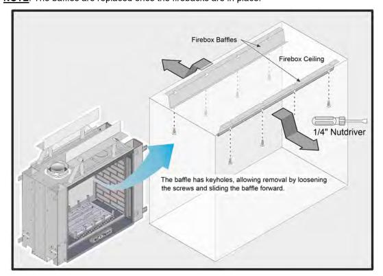
3. Remove the (4) fireback clips (2 on each side) from the ceiling of the fireplace (see illustration below).
