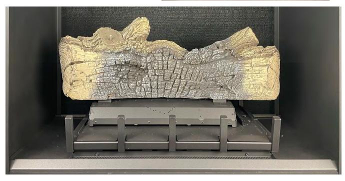
Log #2 has a flat surface on the bottom right branch of the log. The flat surface rests on the firebox floor to the right of the log grate. The left rear of log #2 has a cut-out that rests against the sloped section of the center burner. There are also 2 thin straight grooves in the bottom middle of the log. The right groove rests on the lip of the outer burner. With the log in place, move it back against the center burner as far as it will go.
