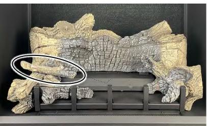
Install log #8 as shown below. The hole on the bottom of the narrow, charred end of log #8 rests on the log locating pin on the right end of log #1. The wider end of log #8 rests on log #2 as shown below.
