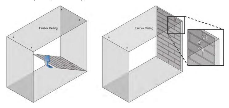
5. Restore the fireplace to the correct configuration (make sure to reinstall the baffles)
