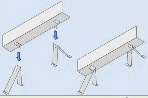
4. Attach the heat shield to the standoffs by aligning the holes on the heat shield tabs with the holes in the header standoffs and secure using the included screws.
